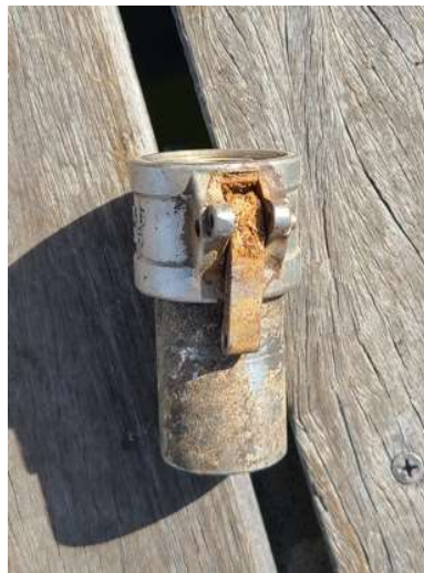
Corroded cam lever
