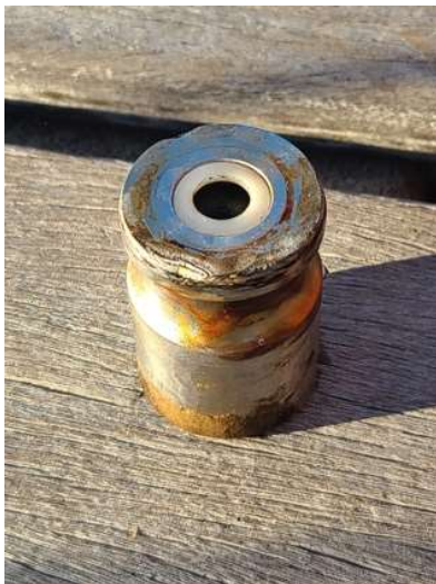
Corroded flow regulator
